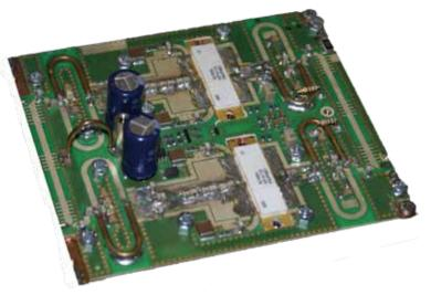
This power amplifier pallet has been designed to cover UHF TV band from 470 to 862MHz and to use in analog and digital applications. UHFAMP500 incorporates microstrip technology and the latest generation of LDMOS power devices from NXP.
