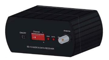
SD-12 is a receiver which can receive audio and data from its transmitter. It supports 7 different frequencies and L&R selection. It has 3 LEDs to indicate if signal level, data or RF are received above limit values. Data and volume can be controlled via its audio transmitter.
