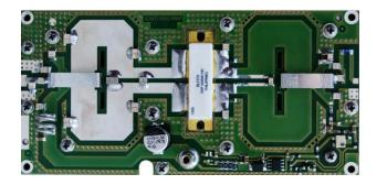
This LDMOS Pallet Amplifier has been designed to operate in the whole FM frequency range (87.5 to 108 MHz), able to deliver max. 800 W output power when fed with 0-2.5 W input power.
