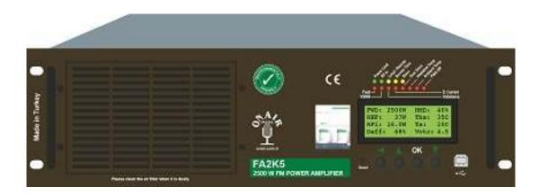
The FA2K5 FM Amplifier is designed to provide more reliable FM transmitters using the extremely rugged LDMOS power transistor for the FM broadcast market.
