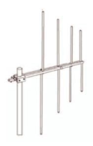
The AT 24/N Directional Antenna is designed for low power transmissions in FM Broadcast Band (87.5 - 108 MHz). This antenna is made with non-corrosive aluminum alloy and composed of four elements and a mounting bracket.
